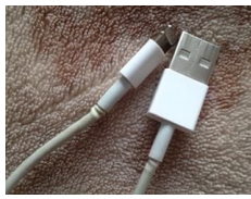
Bends (chins) indicate internal damage
